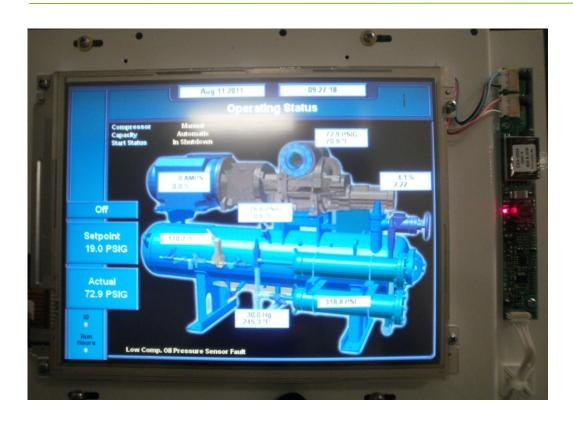
The Display assembly consists of a Sharp LCD screen (model LQ104V1DG61), two fluorescent backlight tubes, a dual backlight inverter module and a wiring harness. The LCD display and the backlight inverter module are controlled by the Quantum 4 processor board.
