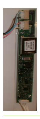
If this voltage is not present, confirm the 12 VDC input to the inverter by carefully measuring across the pins 1 & 4 on connector for the 12 Vdc input (pin 1 is 12VDC, pin 4 is GND). If the voltage is present, the inverter will need to be replaced. If the voltage is not present, contact Frick Service before proceeding.
