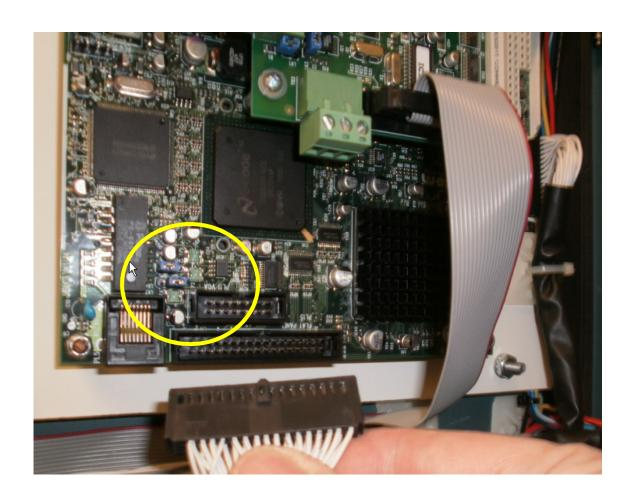
Confirm the proper placement of the backlight voltage jumper LK3 and the display voltage output jumper LK4, on the Quantum<sup>™</sup> 4 processor board. Refer to the Quantum<sup>™</sup> 4 processor board sections of the Quantum LX Maintenance manual for the proper placement of these jumpers for the LDC display being used.
