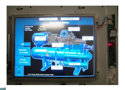
The Quantum LX Sharp LCD display assembly is the operator's visual interface with the Quantum LX Control Panel.
