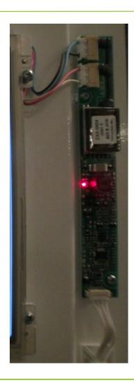
Inspect the harnesses and connectors for possible damage (damaged wires, bent pins, etc.). The display mounting plate will have to be removed from the panel door to gain access to the inverter module.
