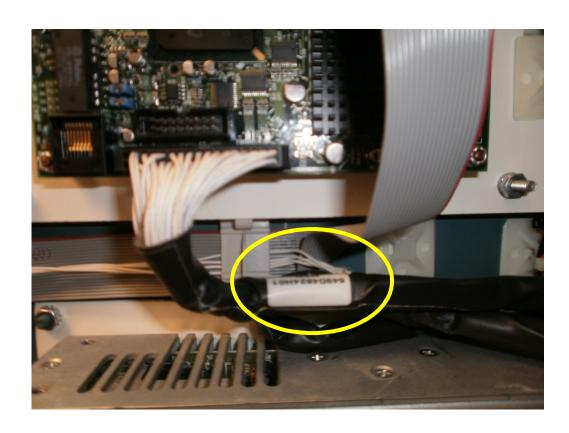
With the Quantum LX power off, confirm that the display and inverter harness is the proper one by part number for the display being used. These cables should have a band around the wires which has the part number written on it. Refer to the Replacement Parts list in the Quantum LX Maintenance manual for the correct part numbers.
