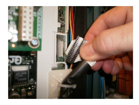
These cables both originate from the same connector, PL15, on the Quantum<sup>™</sup> 4 processor board.
